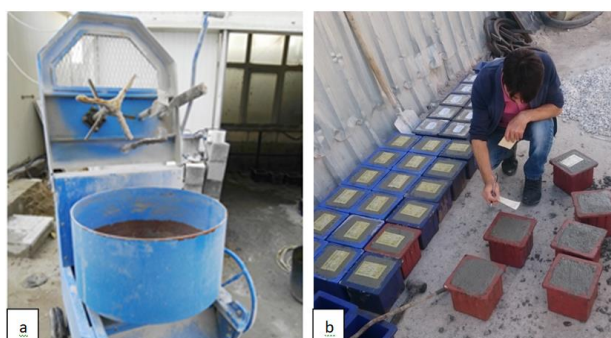
Fig. 2. a) Pan type mixer, b) Molding of specimens
