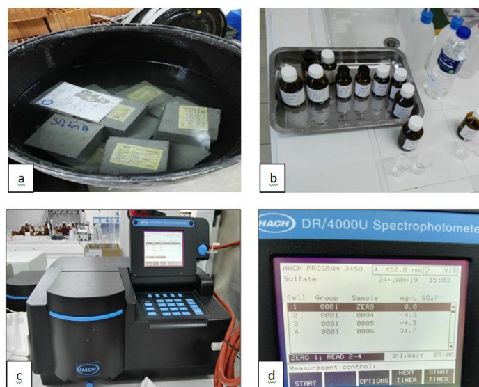
Fig. 3. a) Concrete curing in \text{SO}_4^{2-} solutions, b) Sampling from \text{SO}_4 solutions, c, d) HACH DR/4000U spectrophotometer
