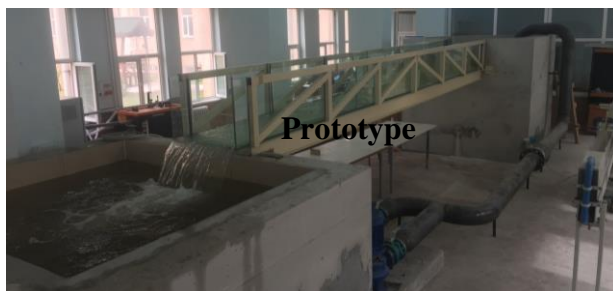
Fig. 3. Open channel systems used as "model" and "prototype"
