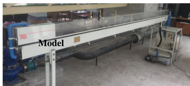
Fig. 3. Open channel systems used as "model" and "prototype"
