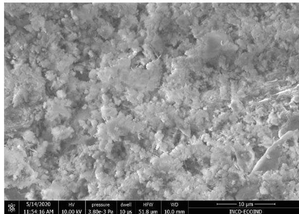
**Fig. 7.** The SEM image of the material obtained from the addition mine tailings (40%) and red mud (10%)
