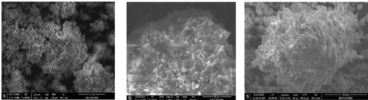
**Fig. 3.** The SEM images for the three component materials of the mortars, a) red mud NR, b) mine tailings S, c) cement C**Table 2.** Experimental variants of mortar mixes
