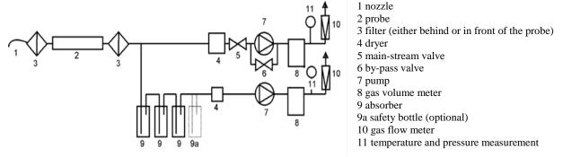
Fig. 2. Schematic of an isokinetic system for air sampling on the filter and absorbent solutions
